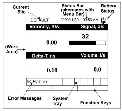
Figure 2-6: The PT878GC Screen in Operate Mode
